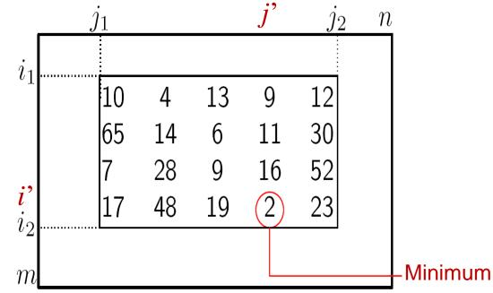
•Input: an  $m \ge n$ -matrix of size  $N = m \cdot n$ ,  $m \le n$ . •Preprocess the matrix s.t. range minimum queries are efficiently supported.
